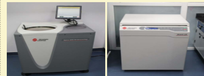
Ultra centrifuge: Beckman Coulter Optima XPN-100 Ultracentrifuge Cold centrifuge: Avanti JE Biosafe cold centrifuge (Beckman Coulter)
