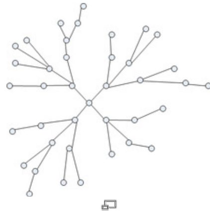
Fig.. 1. Example of how nodes may be interconnected with links to form a telecommunications network
