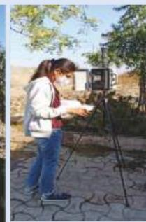
Figure 2: Airmetrics MiniVol Air sampling of Bioaerosols at the study site.
