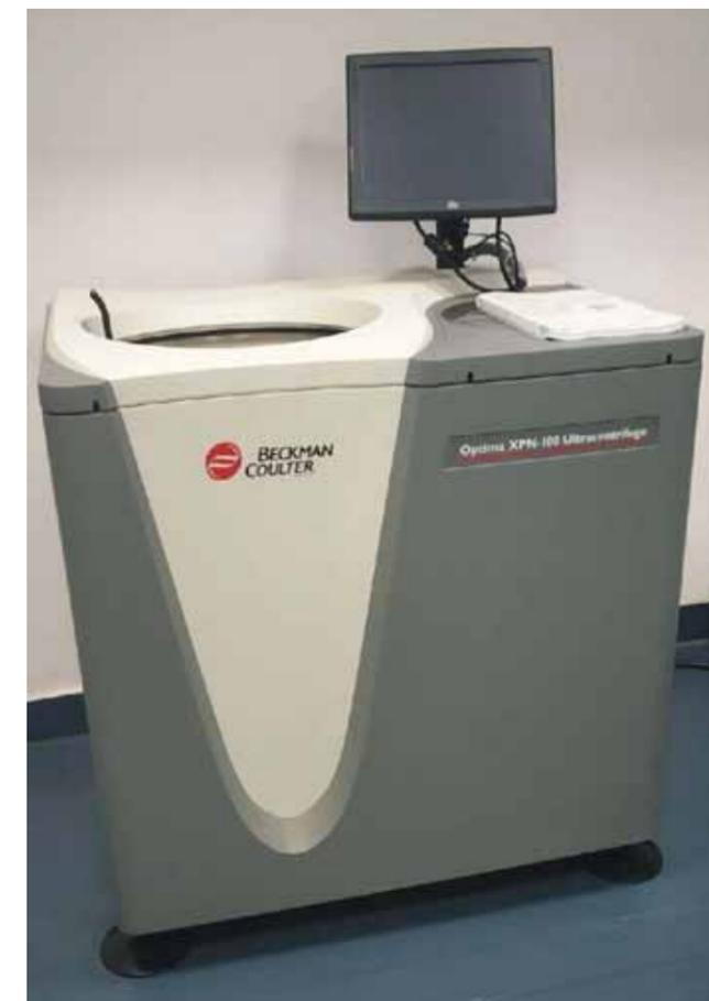
Beckman Coulter's Optima XPN-100 Ultracentrifuge is a high-performance centrifuge optimized for spinning its two rotors at speeds approaching 70,000 rpm and 40,000 rpm (swinging bucket). Maximum speed 100,000 rpm with speed control of  $\pm$  2 rpm of set speed (above 1,000 rpm). Large touch screen display, energy efficient and real time run graphing. Optima XPN boasts additional enhancement that will simplify use, optimize control, security and increase productivity. Ultra-centrifuge offers:
