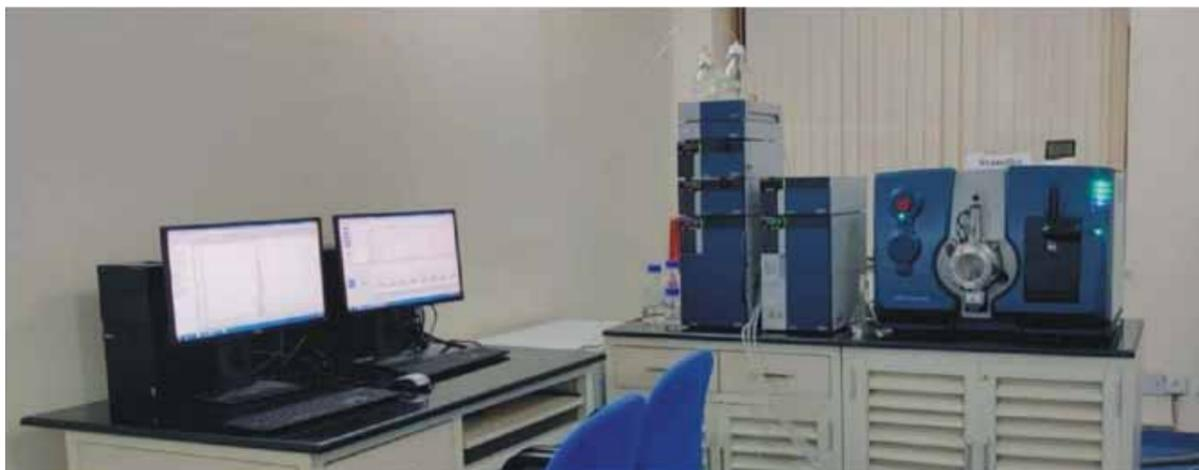
Liquid Chromatography with Mass spectroscopy: a triple stage quadrupole/linear ion trap mass spectrometer, Q-Trap 4500 (SCIEX), equipped with ion sources (turbo V) Electrospray ionization (ESI), and Atmospheric pressure chemical ionization (APCI), autosampler, column oven with HPLC (Exion LC-AC) system. The system is ideal for laboratories requiring ultimate robustness, ruggedness, and reliability for high-throughput screening of many compounds in many samples every day.
