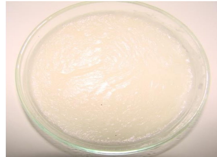
Solvent casting of PHV on modified cellulose
