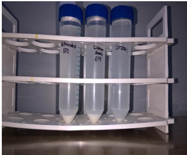
Kaolin test for flocculating activity
