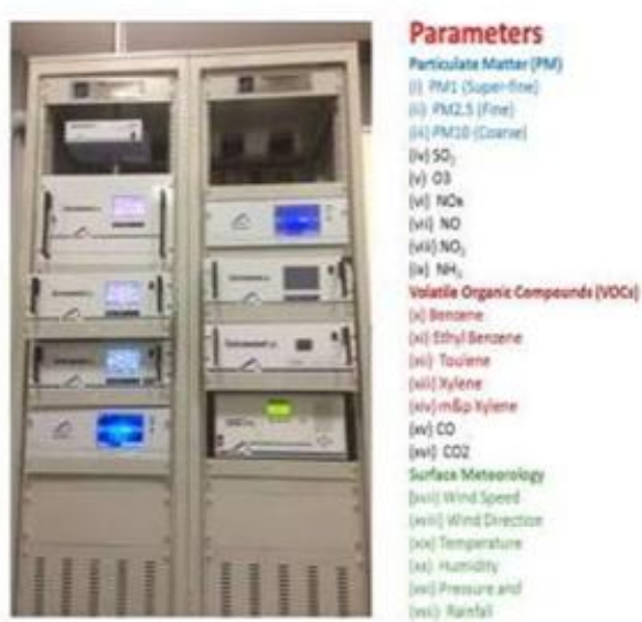
Front-view with data display of the AQMS and rack-mounted PM, Gas Analyzers and
