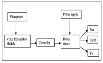
Fig. 5:Block Diagram of Voice Commands
