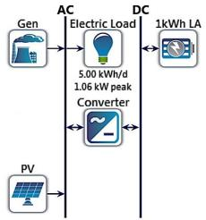
Fig.1. Solar PV Connected Microgrid
