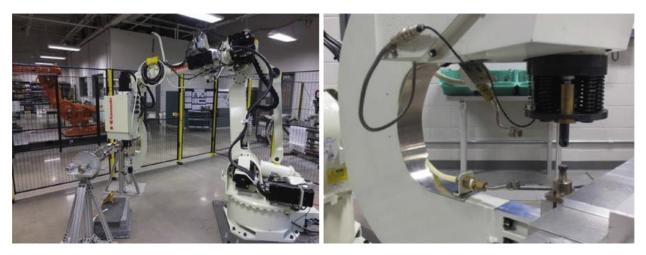
Fig. 2. Kawasaki Robot for FSW
