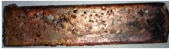
Fig. 4. Casting ingot of developed MMC
