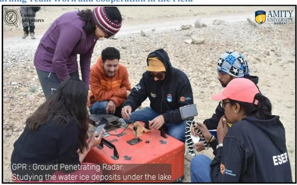
**Ground Penetration Radar: Studying the Water ice deposits under the lake**
